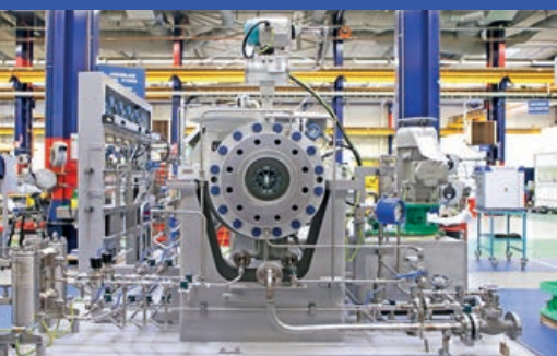
Sundyne compressors boost gas from pipeline pressures to the levels required by turbines.
