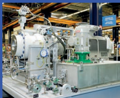
Sundyne compressors boost gas from pipeline pressures to the levels required by turbines.
