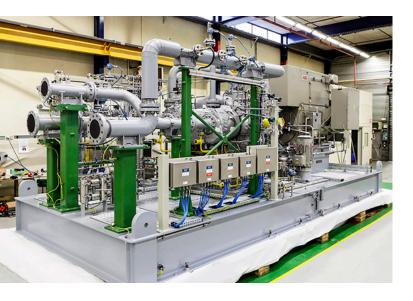
The fuel gas booster is one of the most important pieces of equipment in co-gen power plants, because if the fuel gas compressor fails, the entire power plant stops. Common requirements for fuel gas boosters include: high efficiency across variable suction pressures and several gas turbine
