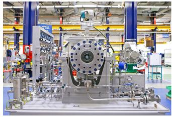
Ever-growing demand for cleaner and more affordable energy is increasing the popularity of gas turbine power generation in industrial and commercial power plants – and most of these plants prefer centrifugal compression to boost fuel gas from pipeline pressures to the higher pressures they require.
